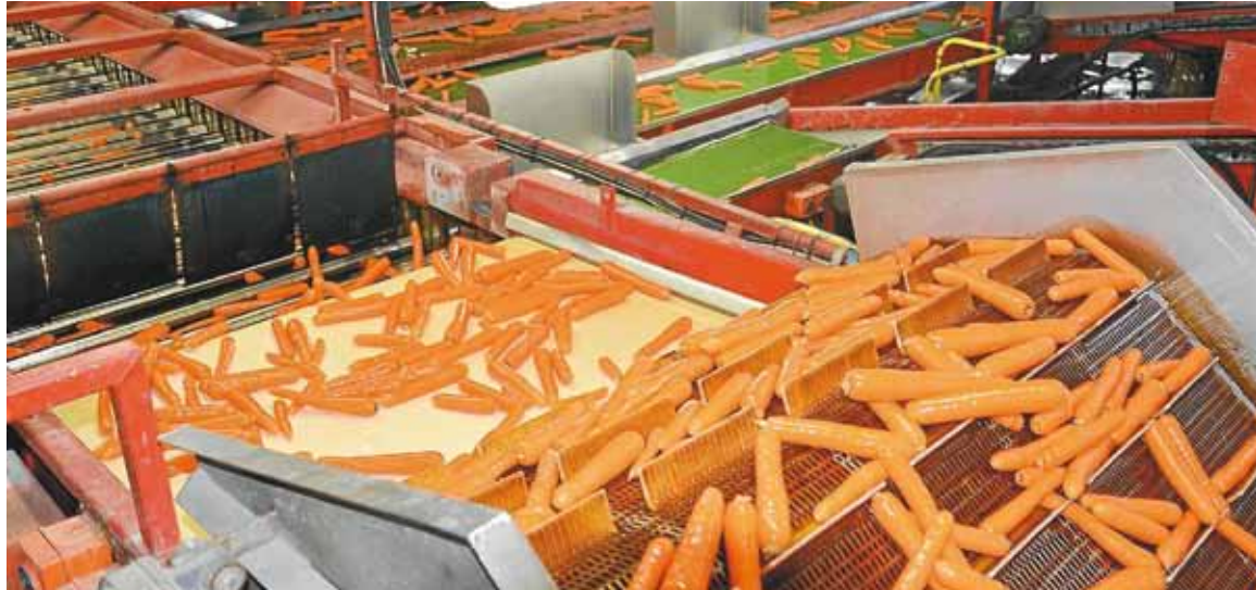
From arrival at the processing facility the carrots are washed, graded, polished, hydrocooled, sized and packed. The packhouse has the capacity to pack 130 tonnes of class one carrots for various markets each day.
