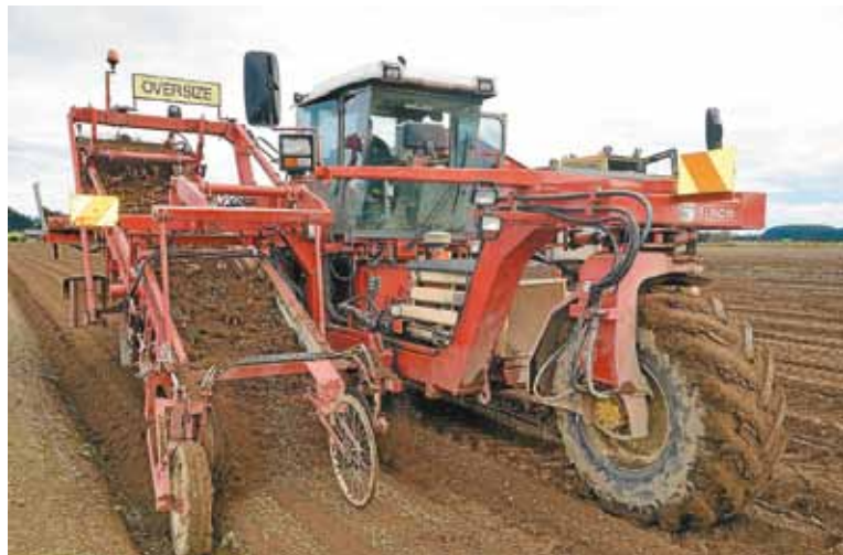
The harvester makes its way through the winter crop with the carrots gently placed into 10t bulk bins to avoid cracking and splitting. It has the ability to harvest 40 tonnes of carrots per hour.
